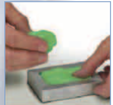
Figure 2: Placing the Objet model inside the mold
