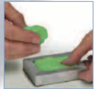
Figure 2: Placing the Objet model inside the mold
