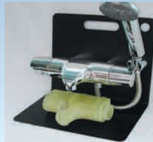
Model before the plating process (photograph – bottom) and model after the plating process (photograph – top)
